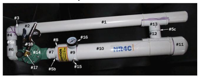
Starting with the barrel, I used a 2 foot length of 1 1/4 inch Schedule 40 PVC from Home Depot as is. The tank was cut from a piece of 2" pipe from Lowes, however, don't cut it yet as it's length is dependant on the overall length of the barrel assembly. Here the pull saw was perfect for the job. You can assemble parts #1, #2 and #3 at this time.
