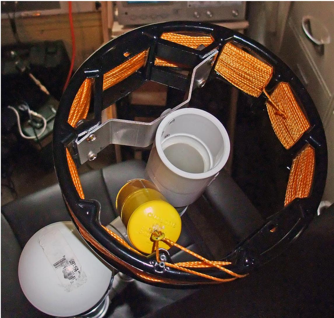
The reel has two plastic fingers that hold the line from getting away before launch. You can make them out if you follow the loop to the missile. Pump up the tank to pressure, attach the reel. Now unwind a turn or two to get some free line and drop the missile in the barrel and reset the line in the fingers to keep it from unwinding. Aim the PAL and squeeze the release lever. It will fire with a noticeable 'crack' in stead of the 'pop' of the
