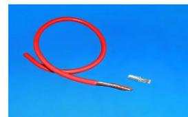
PP contact and crimp or solder in place. I like using the West Mountain Radio ratcheted crimper as it is positive, and quick. Cut the wire about 1 1/2 inches long and repeat until you have seven Red and Black wires with PP contacts attached.
