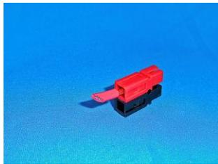
This is a good time to make up the Power Pole connectors. Insert a contact with Red wire into the Red plastic housing. Refer to the cut-away and be sure to orient the contact properly. You
